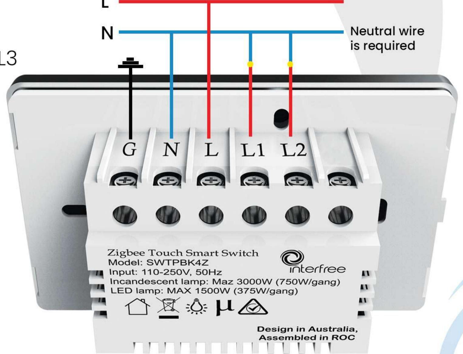
PLEASE NOTE: Please wire up the switch strict accordance with the diagram in the prevention of any damage to the switch. This product must be installed by a qualified electrician.
